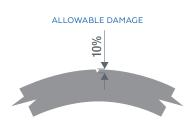
Passing ISO 13479 Notched Pipe Test requires a minimum of 500 hours at 80°C with pressure of 920kPa and a 20% pipe wall notch depth. Millennium® pipe achieves >5,000 hours resistance under these conditions, a factor of ten times that required of conventional PE100 pipe.
