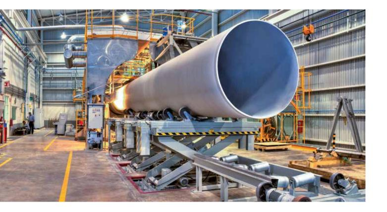
Flowtite® pipes are manufactured using the continuous advancing mandrel process which represents the state of the art in GRP pipe production.
