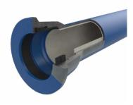
The Jindal SAW manufactured pipe has a socket push-on joint (flexile jointing) with a unique EPDM gasket, clearly identifiable by the green markings on the face of the gasket, allows a guick and safe installation. Due to their high angular deviation, there is the potential to reduce the number of fittings, increasing the rate of installation.
