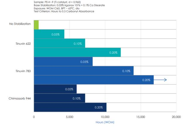
Based on Ciba Specialty Chemicals data, 16000 hours in the Weather-Ometer is approximately equivalent to 12.5 years in Florida. This approximates to more than 10 years of exposure in Australia.<sup>(4)</sup>
