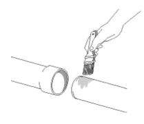
Using a suitably sized brush, apply a thin even coat of solvent cement to the internal surface of the socket first. Solvents will evaporate faster from the exposed spigot than from the socket. Special care should be taken to ensure that excess solvent cement isn't built up at the back of the socket (pools of solvent will continue to attack the PVC and weaken the pipe). Next apply a similar even coat of solvent cement up to the witness mark on the spigot. Ensure the entire surface is covered.
