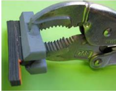
FIGURE 6 – ISO 21751 STRIP BEND SPECIMENT PRIOR TO BENDING
