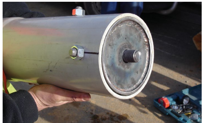
Figure 6.12 Swivel arrangements attached to Restrain™ Sewer Pipe prior to the attachment of a pulling or reaming head
