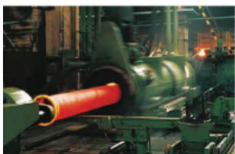
Ironite ductile iron pipe centrifugally cast in machine with water cooled steel moulds
