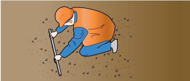
**02** Position the base on the bedding material with a spirit level. Apply Iplex pipe seal lubricant to the pipe spigot and base socket seal for ease of assembly. Connect the base to the pipe by pushing it onto the pipe spigot end.
