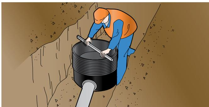
**03** Adjust the pipes to the required position. The adjustable pipe connector enables an angular deflection of 7.5° from the centre line in all directions.
