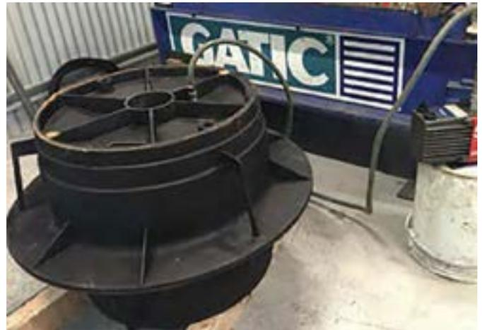
Figure 8: GATIC® EZIpit® 600 'Top Hat' Cover under vacuum test.
