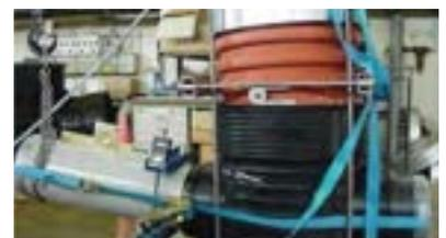
Figure 5: EZIpit® base and corrugated riser under vacuum test with smooth wall PVC pipes
