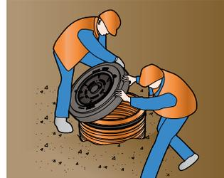
Remove the lid from the cap and apply GATIC® sealing compound liberally to all vertical and horizontal seating surfaces of the lid and assemble on the cap.
