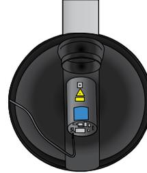
**05** Cut the riser to the required length (refer to 'field height adjustment' Sections 3.4 and 3.5). This is easily performed with a circular saw or handsaw. Cut at the top of the corrugation or in the valley. Remove swarf.
