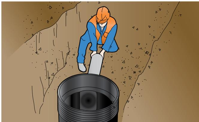
**04** Place the laser inside the base to check the level.
