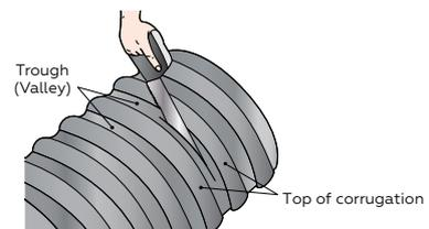
**06** Assemble the sealing rings in the 1st valley at each end of the riser. Ensure the sealing ring is sitting correctly in the valley of the corrugation.
