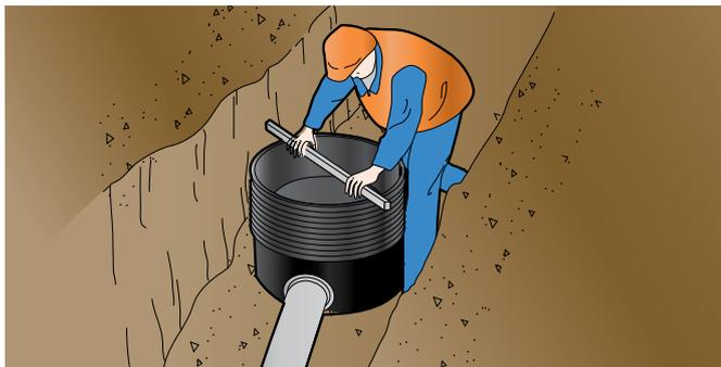
**03** Adjust the pipes to the required position. The adjustable pipe connector enables an angular deflection of 7.5° from the centre line in all directions.
