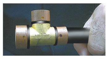
Use the Iplex calliper gauges supplied with the tool to check each and every joint. Gauge tips must fit over the crimped copper sleeve at 90° to the tool jaw split line. Permanently tight connections can only be guaranteed with Iplex approved tools. The tools have to be protected against dirt and damage, and should be cleaned regularly.
