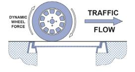
To prevent covers lifting, position covers such that traffic flow direction is from undercut to drawcut.
