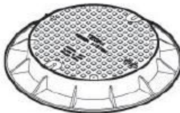
FIGURE A13: DN 600 EZIPIT® FRAME AND ACCESS COVER ARRANGEMENT (CLASS D)
