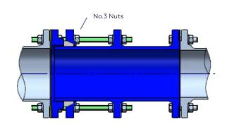
**TYPE 'B' DISMANTLING JOINT COMPONENTS** (THRUST TYPE)
