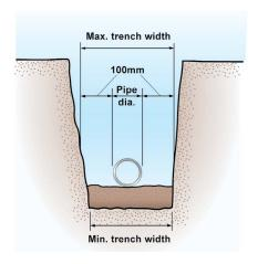
Trenches when excavated are either 'stable' or 'unstable'. The category into which a trench fits is affected by the soil conditions, width, depth and method of excavation. To ensure that maximum support is given to the buried pipe by the undisturbed ground the resultant stable or unstable trench should be treated in the following way:
