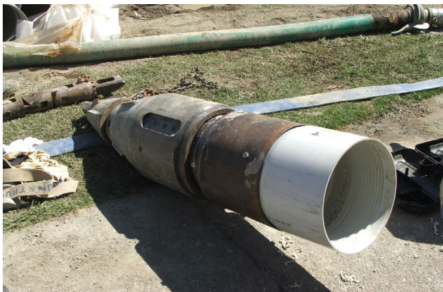
Figure 6.11 Typical external type pulling head attached to the Restrain™ Sewer Pipe
